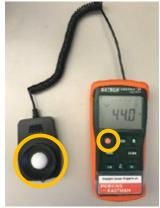
• Confirm that the units on the device are being measured in FC (footcandles) instead of LUX by pressing the bottom right button.
