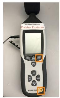
• Set interval to desired number of seconds (45) using the "LEVEL" button. Press "HOLD" button when finished.
