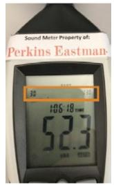
• Press the "REC" button once to start the recording. "REC" should appear in the bottom right corner of the screen. Meter is ready to collect data.
