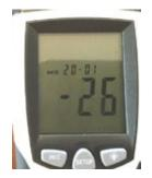
• The next screen should show numbers and nn on the bottom. The numbers represent minutes. Press the "Level" button until the screen reads the appropriate time in minutes. Once there, press the "Setup" button to advance to the next screen.
