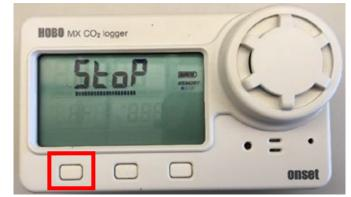
• To offload data from the logger, return back to the HOBOmobile app, connect to the logger, and tap Readout. The data from the logger will be saved to your device.
