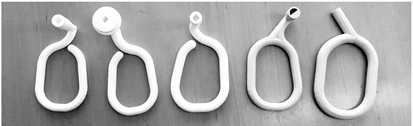
3D printed door handle iterations.
